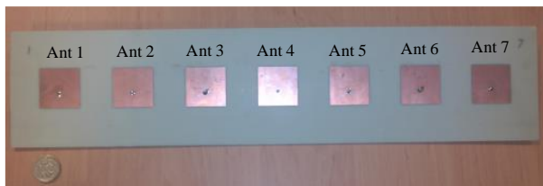
Fig. 5. Front view of the fabricated 1-D 7-element microstrip patch antenna array for 2.442 GHz operation. A ground plane covers the entire back of the board.
